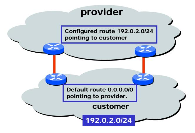
Static routing is the most common way of connecting an autonomous routing domain to the Internet. This helps explain why BGP is a mystery to many ...
