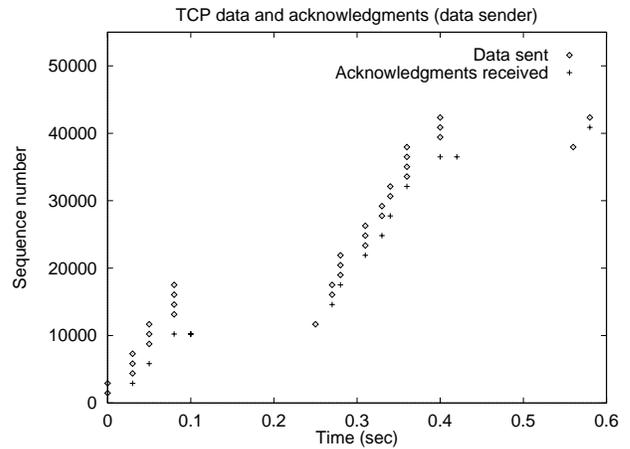
Fig. 5. Scenario 1, TCP trace snapshot (1500 bytes, sender's view)
