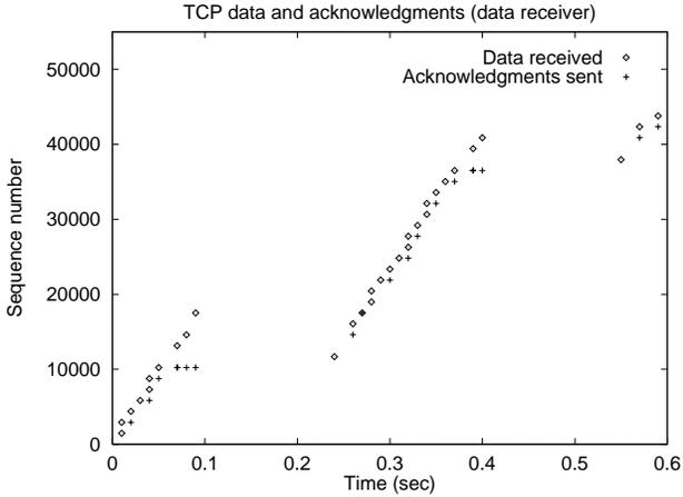
Fig. 6. Scenario 1, TCP trace snapshot (1500 bytes, receiver's view)
